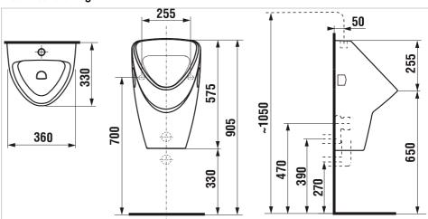
JIKA offers ceramic solutions geared towards the needs of businesses. One of them is Livo, a siphonic urinal with outer water inlet. This urinal can be connected to horizontal or vertical siphon. Antibak prevents trapped dirt by having the inner ring and drains glazed. 100% recyclable. 10-year warranty provided.
