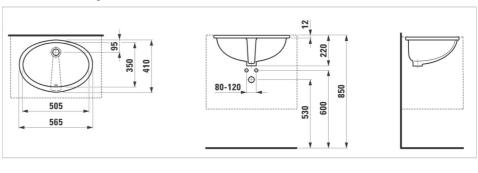
Lipsy washbasin, built-in from underneath, will namely find its place at hygienic spaces designed for the public. Smooth oval shape attached to the washtop from underneath meets the most stringent requirements on both hygiene and aesthetics. For Jika washbasin mounting instructions please see our download documents. An extended 10year warranty is provided for all JIKA ceramic products!
