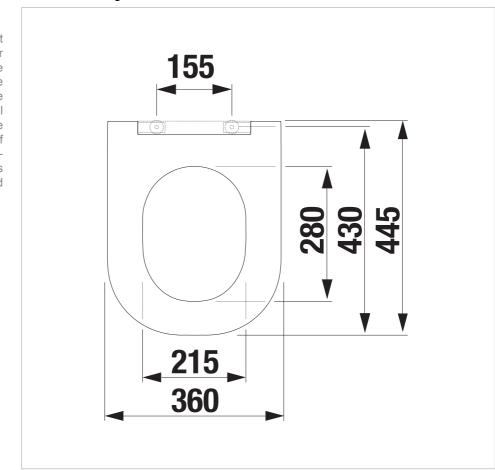
Thin, easy-to-remove Mio-N duroplast seat and cover meets all requirements for a modern product. High-quality, durable and dimensionally stable material, simple yet elegant and practical shape of the seat, complemented by stainless steel hinges and an ingenious Slowclose mechanism that slows down the folding of the seat. The seat is suitable for the wall-hung toilet Mio-N. This year's novelty is the new color design black matte and white matte. Available 1Q 2024.
