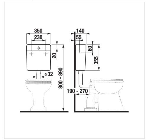
Modul plastic cistern is an elegant solution for free-standing toilets. We offer it with a 3/8" side water supply including a elbow for connection to the toilet and Start-Stop flushing.
